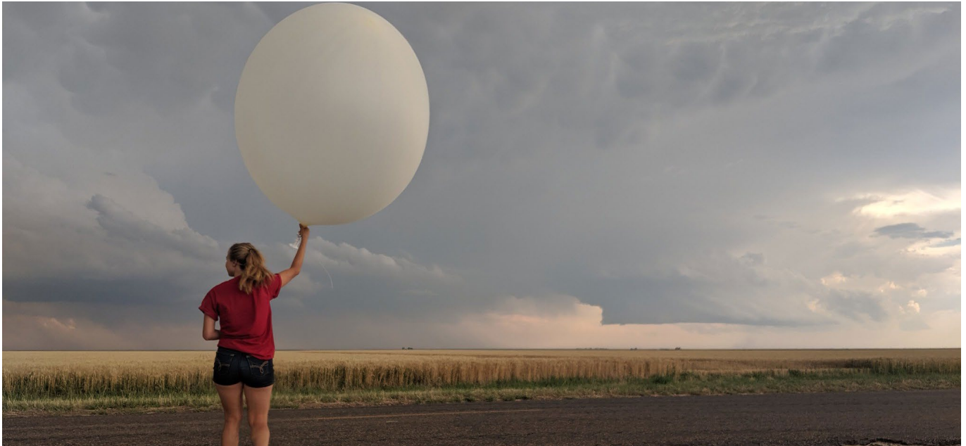
The NOAA NSSL Windsond researcher launch balloons that are smaller than normal weather balloons, with up to eight in the air at once. (Photo by Christiaan Patterson (OU CIMMS/NOAA NSSL))
